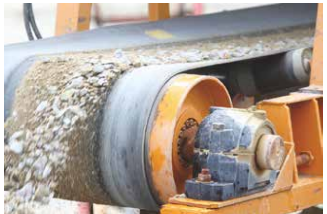
SIT-LOCK® 1 used for a conveyor belt pulley.
