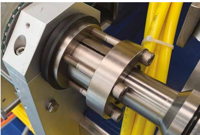
Locking two shafts using SIT-LOCK® 10, nickel-plated version.
