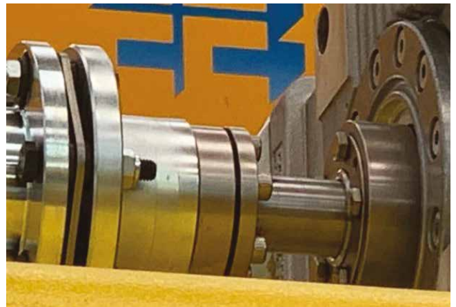
SIT-LOCK® 3 used for a disc coupling.
