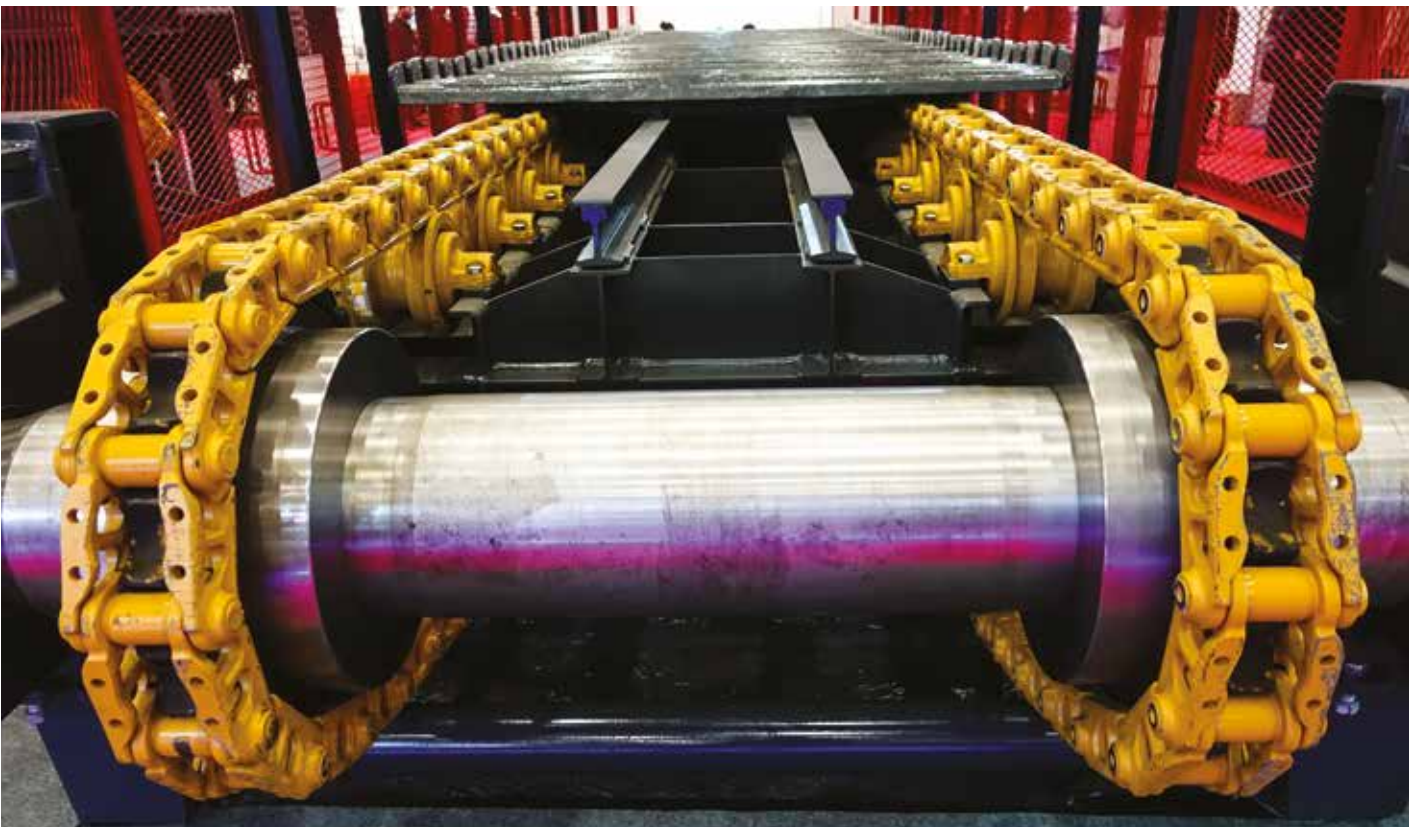
Locking conveyor chain wheels using SIT-LOCK® 4 COMPACT.
